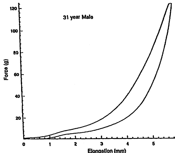
Figure 9. These are stress-strain curves of human vocal ligaments. 9A (upper left) is a 61 year old male. 9B (left) is the same 61 year old male with functions of elastin and collagen drawn in. 9C (above) is a 31 year old male for comparison with the 61 year old male.
